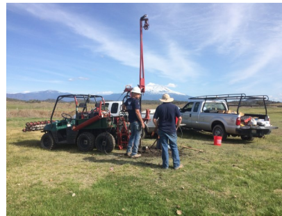
Drilling a piezometer well
